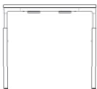
Linear-Fuß: Variable Höhe, Schraube, 62-92 cm Straight leg: Variable height, screw, 62-92 cm
