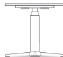
T-Fuß: Variable Höhe, Elektro- motor, 65-130 cm T-leg: Variable height, electric motor, 65-130 cm
